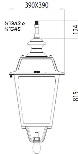
FIRENZE EVO S Suspended installation 1/2" GAS o 3/4" GAS L=124mm fixing type
